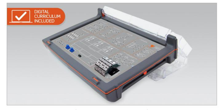
The 3-Phase Control Systems Trainer is a rugged, self-contained hardware unit that enables students to investigate practically and safely the generation of a 3 Phase supply and operation of a Motor and Inverter. The self-contained unit also incorporates three supply transformers.
