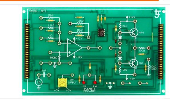
This electronics study card is designed to connect to the 409-01 Experiment Platform or to the 300-01/300-02 Advanced Electronics Experiment Platforms\* as part of a modular electronics programme.
