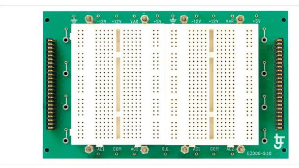
This electronics study card is designed to connect to the 409-01 Experiment Platform or to the 300-01/300-02 Advanced Electronics Experiment Platforms\* as part of a modular electronics programme.
