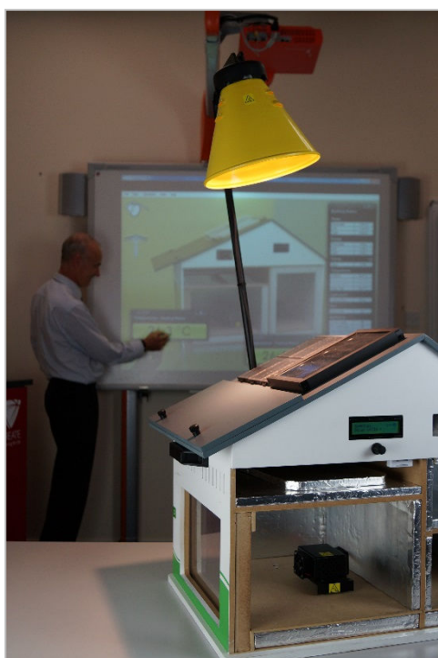
Eco-house – Controlled and monitored via a computer and whiteboard
