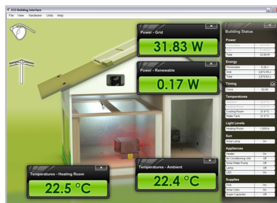
Example – Showing power usage and temperatures in the eco-house
