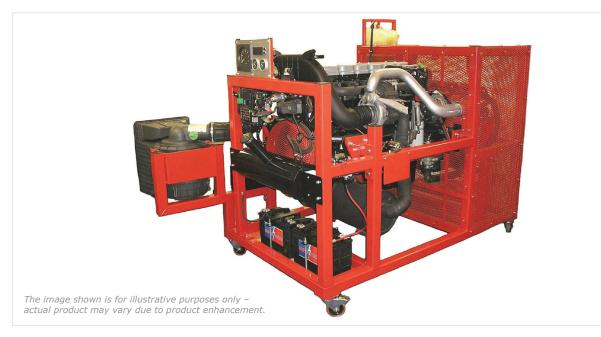
This trainer provides the instructor with a complete working 4-cylinder heavy vehicle diesel engine with a Bosch EDC engine management system and high-pressure common rail fuel injection system. A 6-cylinder version is also available.
