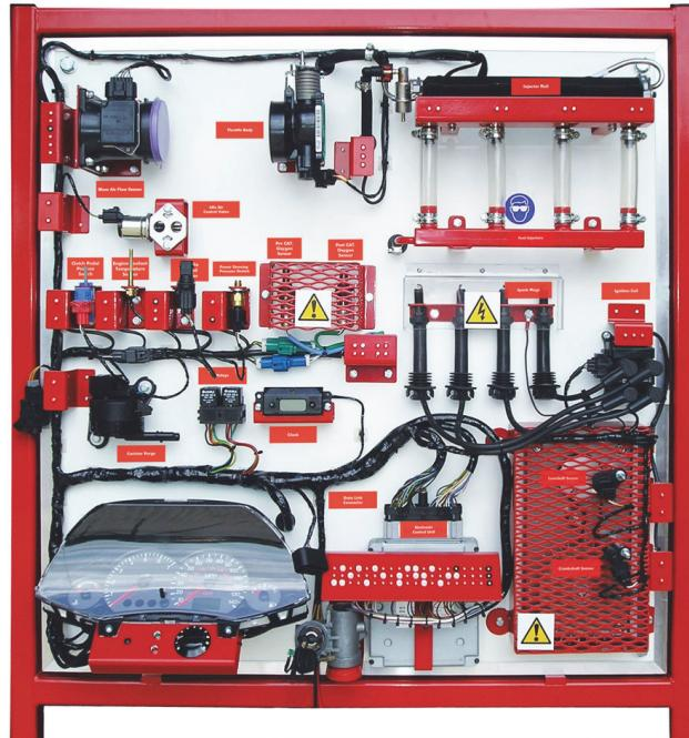
This real component trainer provides the instructor with a working multi-point fuel injection system for group or whole-class demonstration.
