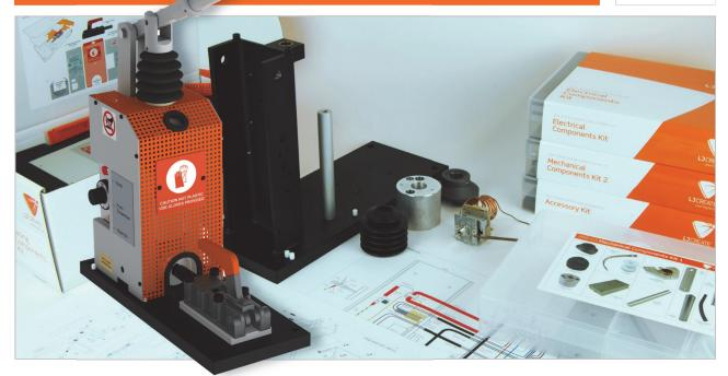
The Mechanical Maintenance - Molder Assembly Kit contains a set of parts and associated instructions - to provide students with an opportunity to learn and practice the hand skills required for maintenance of mechanical and electrical equipment.
