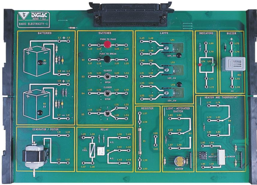
This electronics study module is designed to connect to the Advanced Electronics Experiment Platform (300-01) as part of a modular electronics programme.
