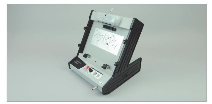
This unit provides power supplies and connection facilities for the complete range of advanced electronics circuit boards.
