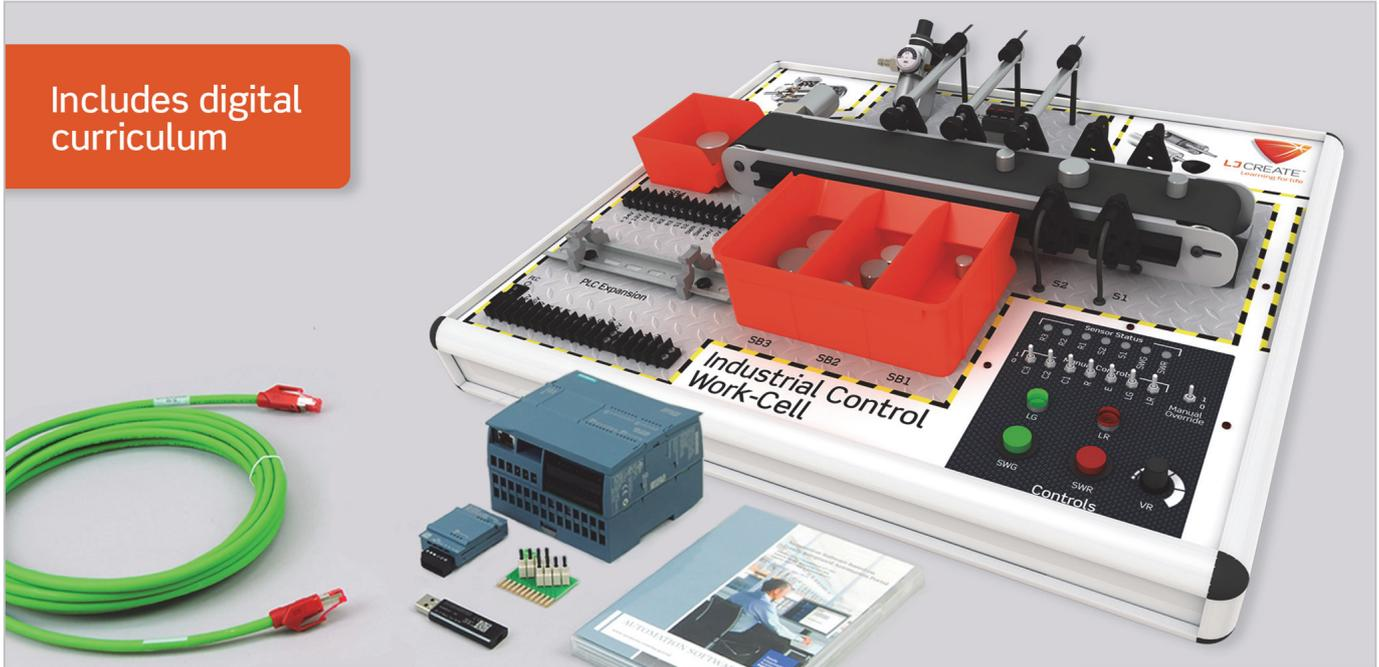
This training system offers a platform that enables students to perform a comprehensive range of PLC programming tasks using a Siemens controller and a conveyor belt/pneumatic sorting application.
