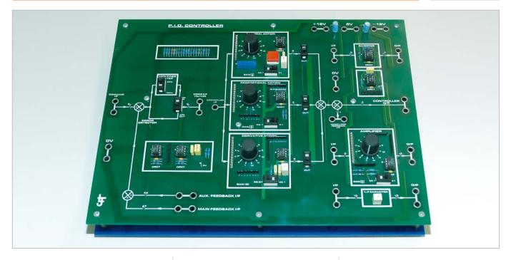
The 207-04 PID Controller module is an analog control system that allows the investigation of three-term control actions which can be configured in conventional servo or process modes.
